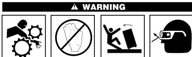
**Do not wear gloves or loose clothing when operating Power Drive. Keep sleeves and jackets buttoned. Do not reach across the geared threader.**
