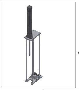
Master-Lee Engineered Products Inc. has come up with two more options for pushing and pulling the flux thimbles. The first option is a hydraulic tool that is capable of pushing or pulling the flux thimble one foot. This tool locks to the seal table similar to the Master-Lee Jacking Tool. The picture on the left is of the hydraulic tool. Which consists of the tool, hoses, fittings, hydraulic oil, and a manual hydraulic pumper.
