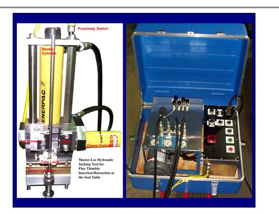
The Master-Lee Flux Thimble Tube Jacking Tool is used at the seal table to assist with removal and installation of flux thimble tubes during outages. The system consists of a Portable Jacking Tool, Control Console and Hydraulic Power Supply. The 115 vac Hydraulic Power Supply and Control Console are mounted on a movable upright cart to facilitate ease of movement throughout the containment building.
